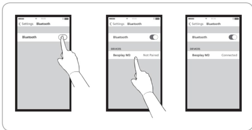
**EN** Beoplay M3 is a connected speaker, using Google Chromecast built-in Multi-room and Apple AirPlay. As a point-to-point source, Bluetooth is always open for pairing. Turn on Bluetooth on your device and select Beoplay M3.
